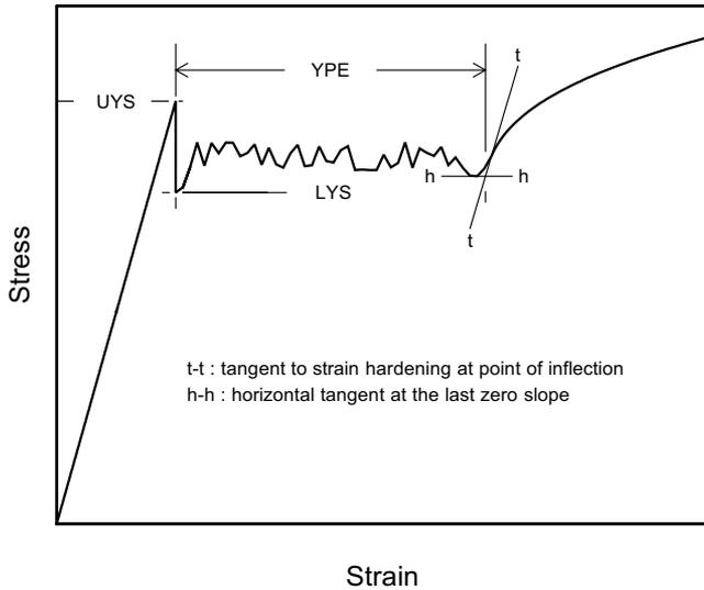
**FIG. 23 Stress-Strain Diagram Showing Yield Point Elongation (YPE) and Upper (UYS) and Lower (LYS) Yield Strengths**
