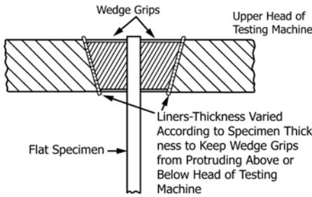
FIG. 2 Wedge Grips with Liners for Flat Specimens
