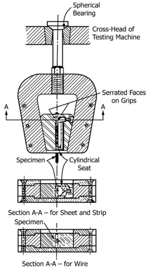
FIG. 5 Gripping Devices for Sheet and Wire Specimens
